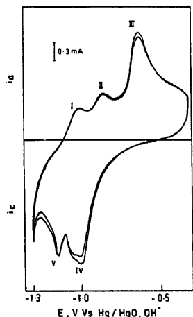
Fig. 1. Typical cyclic voltammogram for solid iron electrode in 5.35 M KOH + 0.65 M LiOH solution. Sweep rate = 20 mV sec -1 , E 1c = -1.3 V and E 1a = -0.3 V.
